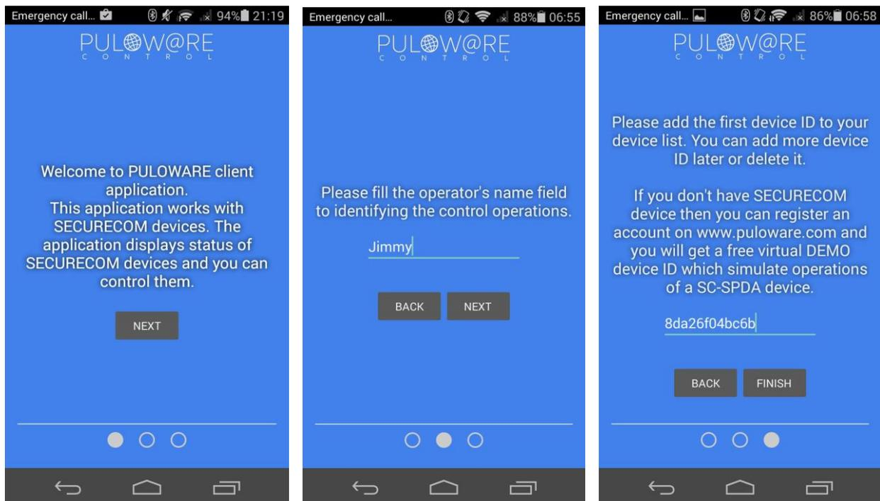
This 16-digit combination of letters and numbers can be found on the sticker, placed on the bottom of device. After the number is typed in, you can finish the setup. If you want to add more devices to the same application, use the „+” sign on the top of screen. This application can be used to handle more than one device, other devices (different device types as well) can be added within the application.
