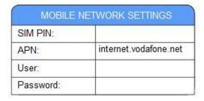
The APN configuration of the SIM card with mobile internet capability necessary for remote configuration and the use of mobile application and the PIN code (if the card is protected by PIN code) of the inserted SIM card can be entered here.
