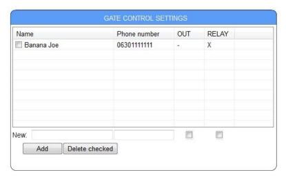
The telephone numbers set here are authorized to remote control the output or outputs assigned free of charge, since in case of calles initiated from the phone number specified here the intercom performs the control and does not take the call but rejects it. Maximum 100 user phone numbers can be added.
