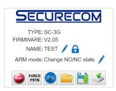
Here you can **RESTARTING** the SC-3G communicator, **FORCE to PSTN** mode the device (switch the incoming PSTN line directly to the alarm panel, so it can receive modem calls), **SWITCH** the **OUTPUT**, **LOAD** settings file, **SAVE** the current settings to a file, and **DOWNLOAD** the current settings that are presented on the page ( when you make some changes in setting) to the device. Also, here you can **ADD NAME** to the device and select the open collector output **ARMED** mode.
