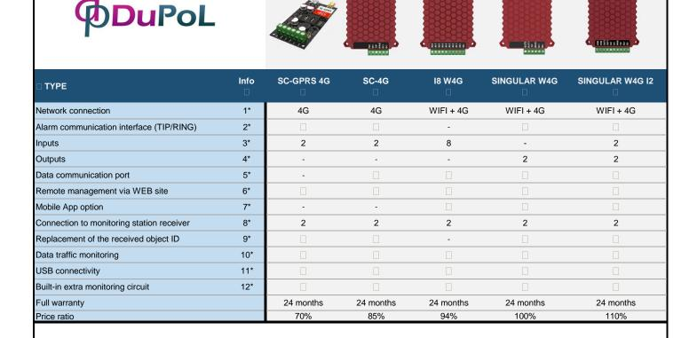
1\* The communicators are able to communicate on LTE Cat1 standard, i.e. they can use the full 4G data service available on all networks. There is no need for a special data network SIM card as is only required for CAT-M and NarrowBand IoT network capable devices.
