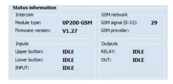
Displays information about the switching state of the peripheries and the actual status of the mobile network.
