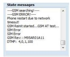
The messages shown in this window give information about the internal operation of the unit. This helps in identifying an internal process, an incorrect configuration or other malfunction.
