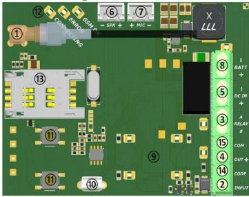
**INPUT, CODE** inputs and **OUT+** output are defined to the COM common negative point, so they need to be installed in pair with COM cable.
