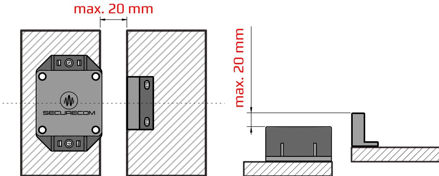
Moving the magnet closer or further away from the device, i.e. opening or closing the gate will cause the blue LED on the unit to flash. (this is visible under the cover plate in low light conditions)
