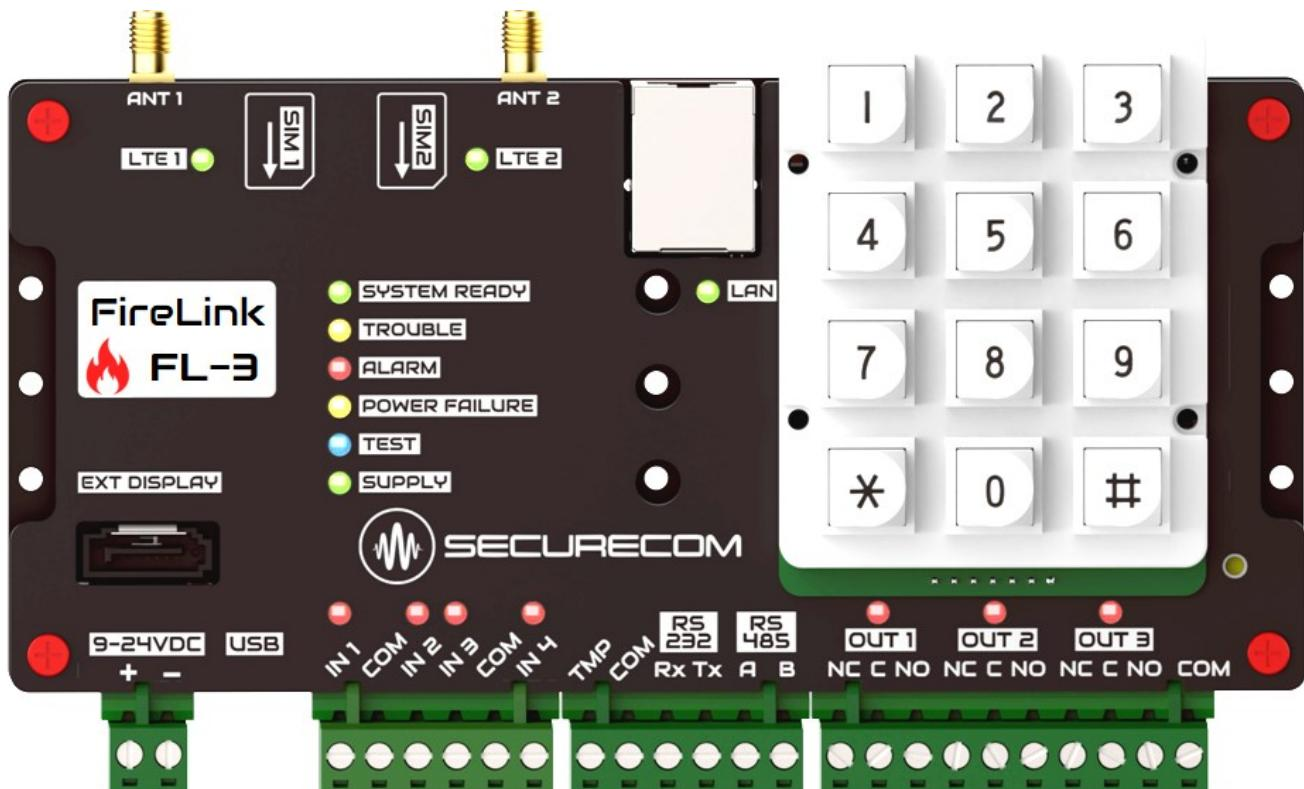
The FireLink FL-x transmits signals of fire alarm control panels to monitoring station. It generates events from contacts received on its inputs from the connected fire alarm control panel. The events are transmitted in a duplicated way to the monitoring receiver through its two independent modem units.
