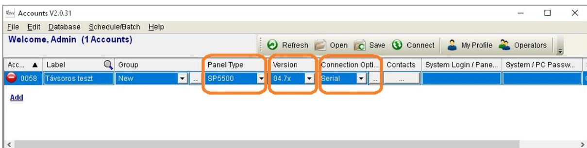
Panel Type: e.g. SP5500 (the alarm panel tested in this specification)
